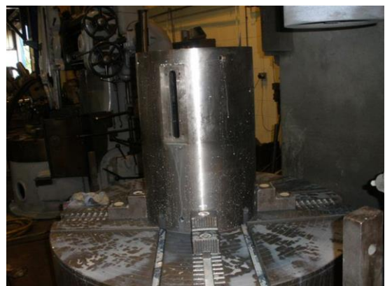
CH-70 Cylinder Getting Finish Ground
