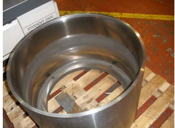
Packing sleeve hard faced in Ni, Cr.
