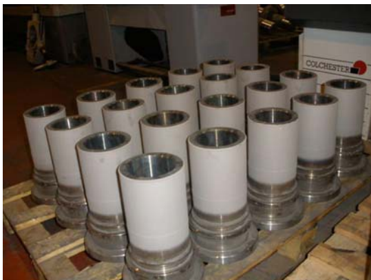
Washpipes coated in Colmonoy-88 (Ni,Cr,B,Wc)
