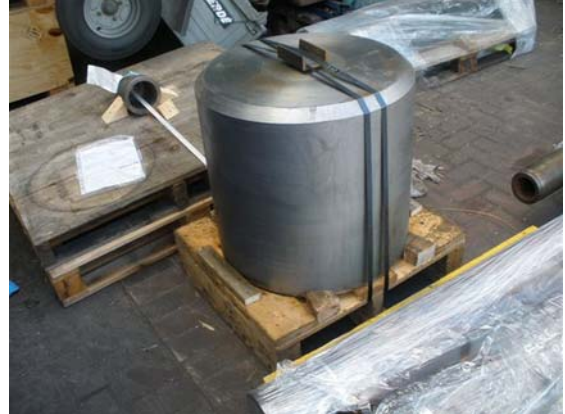
Main ram in for coating and grinding
