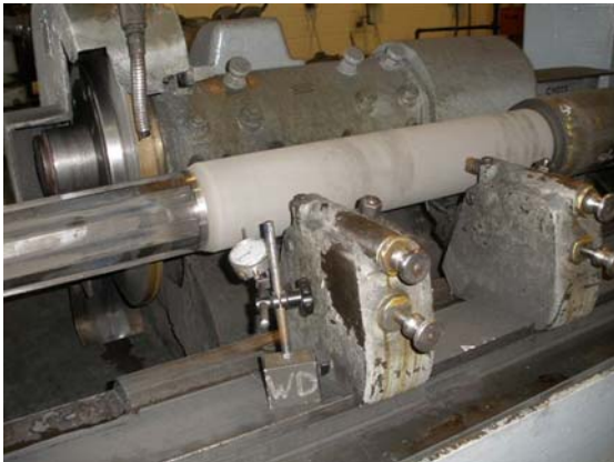
Splined mandrel coated in 1086 (Wc,Co,Cr)
