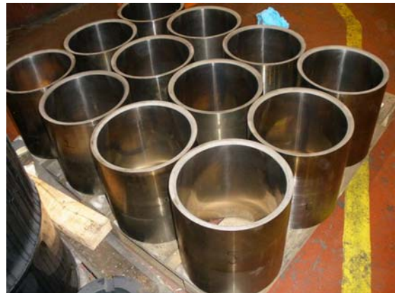
VB Cylinders sprayed and ground in 1060 (Ni,Cr,B.)
