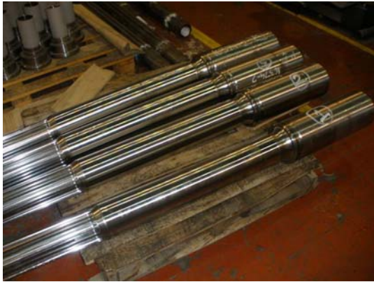
Splined mandrels prepared for coating
